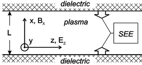
Fig. 1. Schematic diagram of the simulated plasma system. Two dielectric walls represent the coaxial ceramic channel of a Hall thruster.
