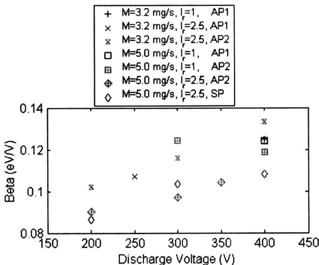
FIG. 3. Linear fit parameter  $\beta$  for several discharge voltages, mass flow rates (M), inner to outer magnetic coils current ratios ( $I_r$ ), and probe design (AP=unshielded alumina probe holder, SP=segmented graphite shielded probe holder) (see Ref. 7).
