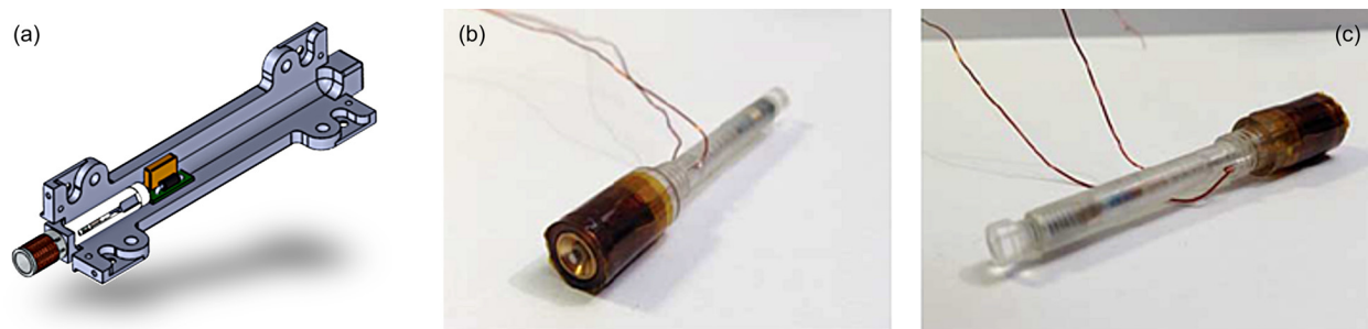
FIG. 16. A schematic of the thruster head mounted in a CubeSat Rail (a), and pictures of a thruster head [(b) and (c)]. In a vacuum arc, the discharge is initiated on the cathode surface. Plasma is generated depending on the material and surface structure in so-called arc spots. These micro-plasmas expand into the vacuum and allow current to flow directly from the cathode to the anode along a lower resistance plasma discharge path.
