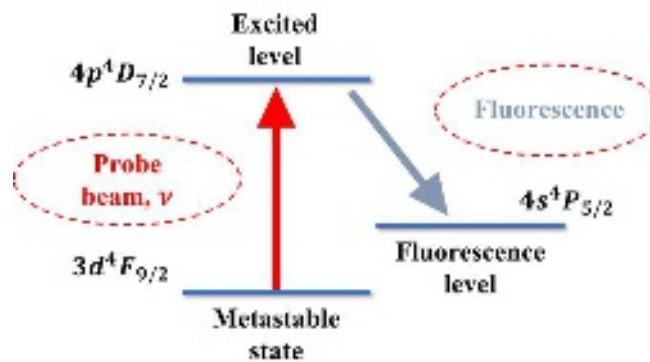
FIG. 7. LIF transition for Ar-II (argon ion).
