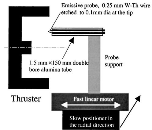
FIG. 5. Schematic of the fast emissive probe setup.
