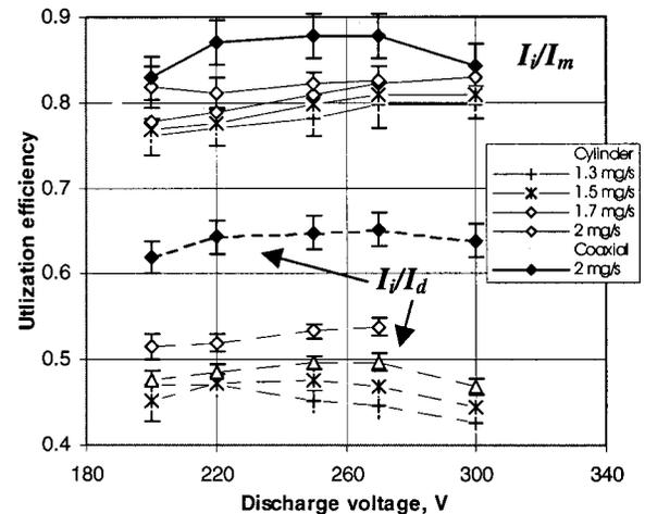
FIG. 13. Propellant utilization,  $I_i/I_d$ , and current utilization,  $I_e/I_d$  of the cylindrical thruster. Note comparison to the coaxial Hall thruster. The propellant utilization does not include the cathode flow rate of about 0.2 mg/s.
