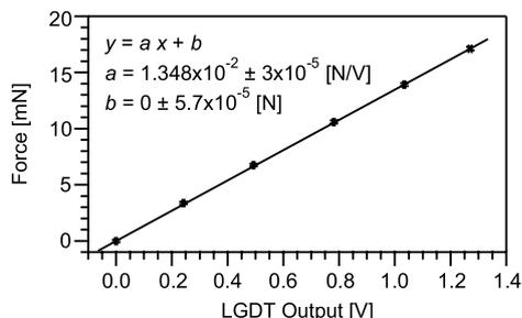
Fig. 2 Applied calibration force plotted as a function of LGDT response. The linear curve is a fit to the displayed data. Error bars on the data points and the fit coefficients represent a 68% ( $1\sigma$ ) confidence interval.
