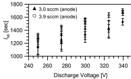
**Fig. 5**  $I_{sp}$  as a function of discharge voltage. The error bars represent a 95% ( $2\sigma$ ) confidence interval.
