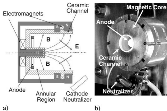
Fig. 1 PPPL cylindrical Hall thruster: a) schematic illustration and b) photograph.
