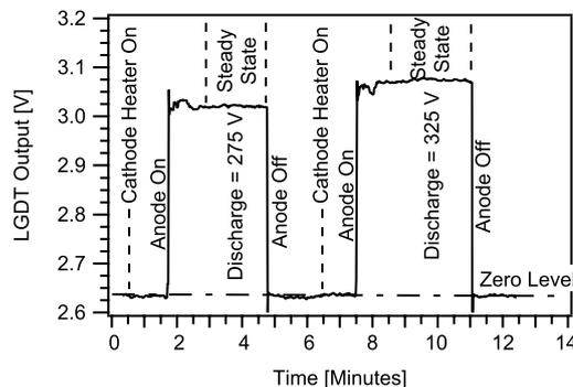
Fig. 3 Raw LGDT output data as a function of elapsed time for two thruster operating points.
