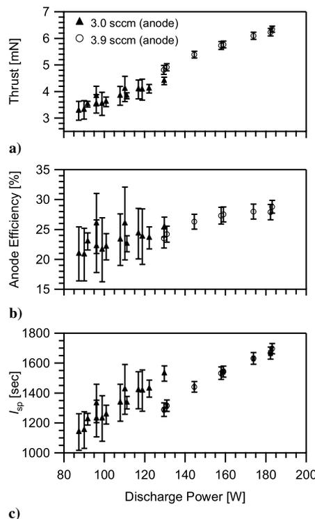
Fig. 4 Performance measurements for a 3-cm cylindrical Hall thruster: a) thrust, b) anode efficiency, and c)  $I_{sp}$  as a function of discharge power. The error bars represent a 95% ( $2\sigma$ ) confidence interval.
