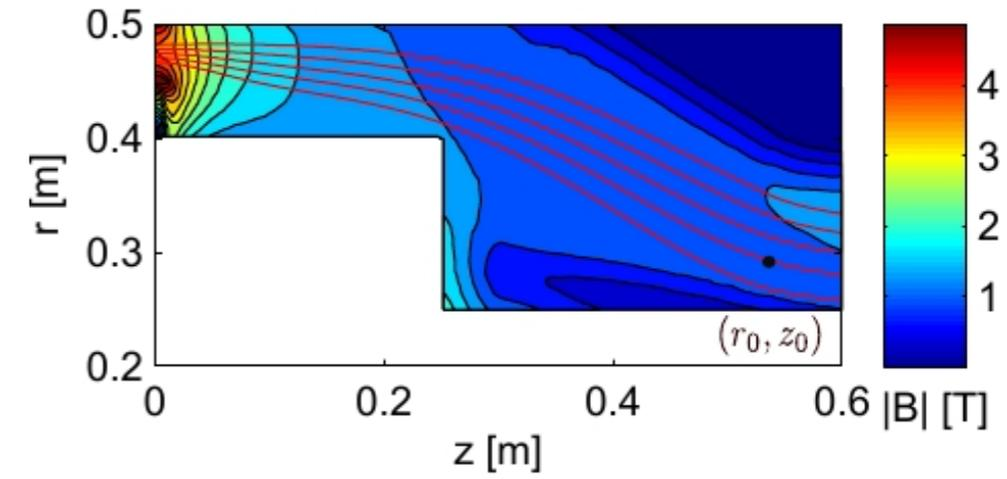
Magnetic field map used as a simulation input, and ion (144 amu) trajectory in the 3D field with collisions (<sup>241</sup>Am).
