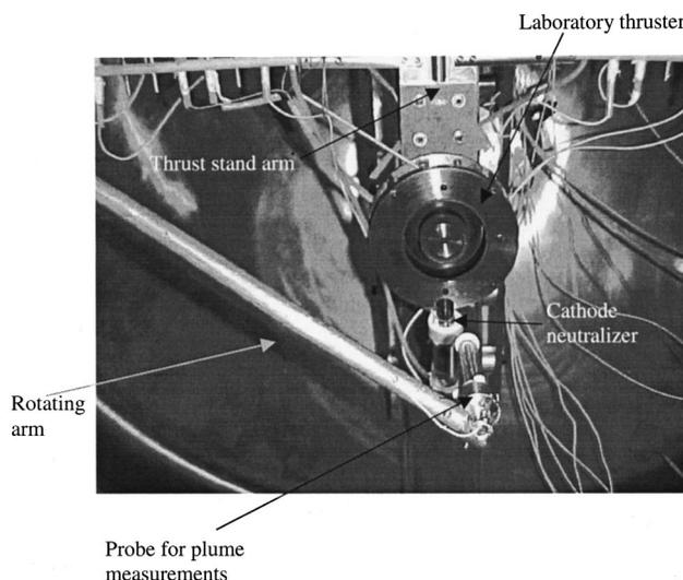
FIG. 2. PPPL segmented electrode Hall thruster.
