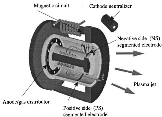
FIG. 1. A schematic drawing of Hall current accelerator with two segmented electrodes.  $E$  is the accelerating electric field,  $B$  is the applied magnetic field, and  $I_H$  is the electron Hall current.
