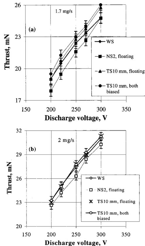
FIG. 6. Thrust vs discharge voltage at the anode mass flow rates of 1.7 (a) and 2 mg/s (b) measured for accelerator configurations with two segmented electrodes, one segmented electrode (NS) and without segmented electrodes. The thruster efficiency was estimated with taking into account the mass flow rate through the cathode.
