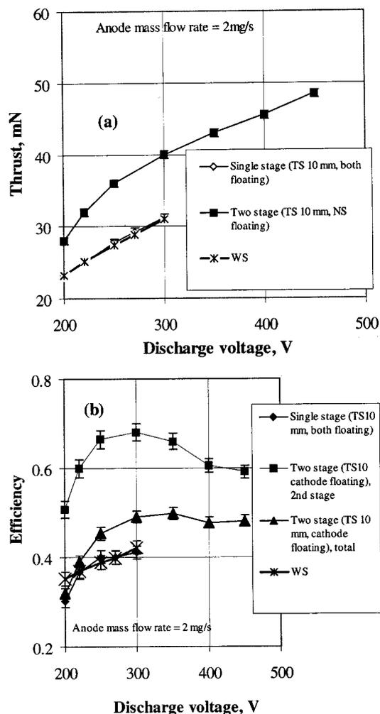
FIG. 10. Thrust (a) and the efficiency (b) vs discharge voltage measured for a two stage accelerator configuration at a mass flow rate of 2 mg/s and their comparison with conventional thruster configuration without segmented electrodes and with two segmented thruster configuration for 10 mm spacing between electrodes.
