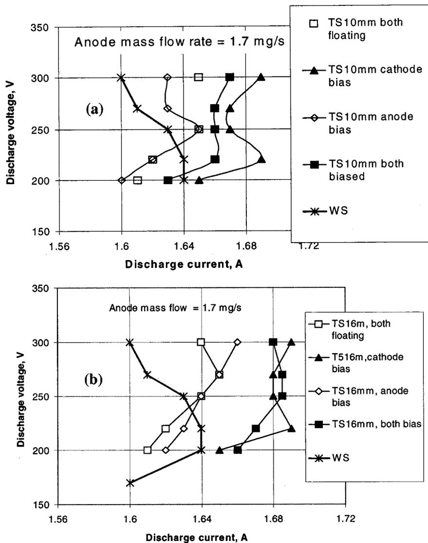
FIG. 4. Discharge voltage vs discharge current at 1.7 mg/s for 10 (a) and 16 mm (b) spacing between the segmented electrodes. TS is "two-segment" case, WS is "without segment" or conventional Hall thruster case.
