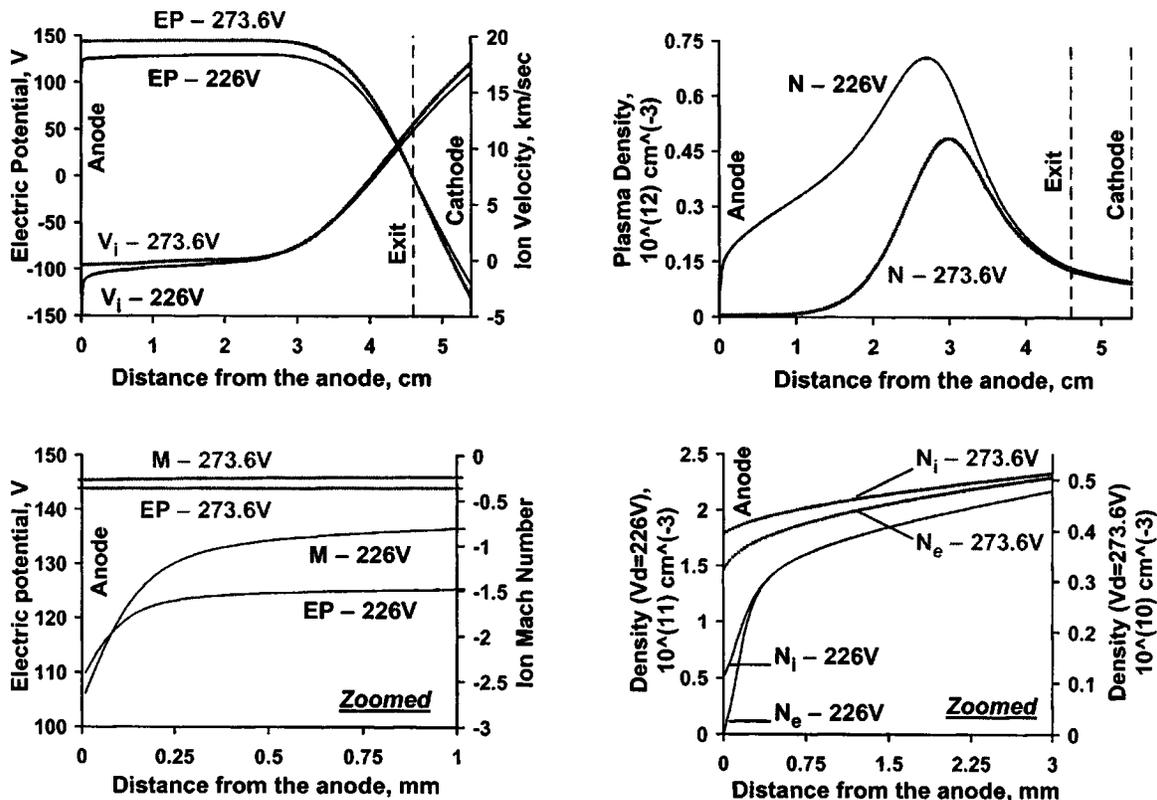
FIG. 2. The numerically obtained electric potential, (EP), ion velocity ( $V_i$ ), ion Mach number ( $M$ ), plasma density ( $N$ ), electron density ( $N_e$ ), and ion density ( $N_i$ ) profiles for  $\dot{m}=1.7$  mg/s and two discharge voltages:  $V_d=226$  V and  $V_d=273.6$  V. The bottom charts are focused on the near-anode region.
