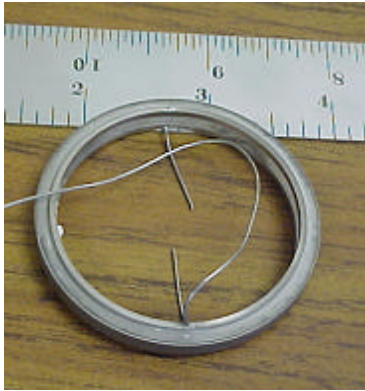
Fig. 4 Emissive segmented electrode constructed from a dispenser tungsten ring with a heater filament incorporated inside the ring and insulated by a sintered ceramic material.
